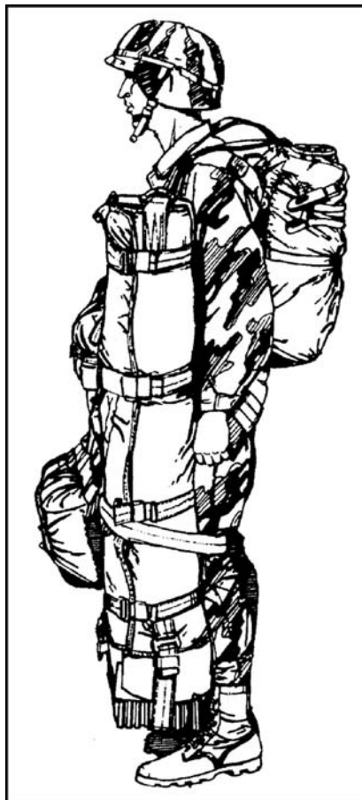
Figure 12-59. Lower tie-down tape routed around AT4JP.
